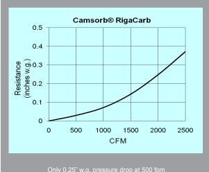
Camfil Farr's CamSorb RigaCarb will improve indoor air quality by controlling offensive and nuisance odors. The CamSorb RigaCarb deep pleated filter is manufactured from familiar Camfil Farr Riga-Flo components, and is designed to fit anywhere a Riga-Flo, or headered style Riga-Flo can be installed.
